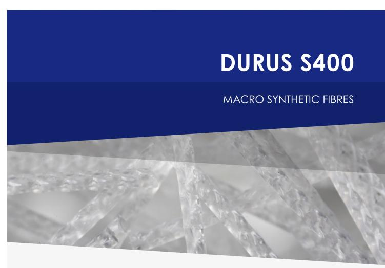
Durus \$400 is a macro synthetic fibre that is extruded, embossed and then specifically cut into the lengths required for each concrete application. Durus \$400 is used in ready mixed, precast and sprayed concrete in both above and in underground applications. The embossment improves the bond between the fibre and the concrete resulting in improvements to the residual flexural strength of the concrete.
